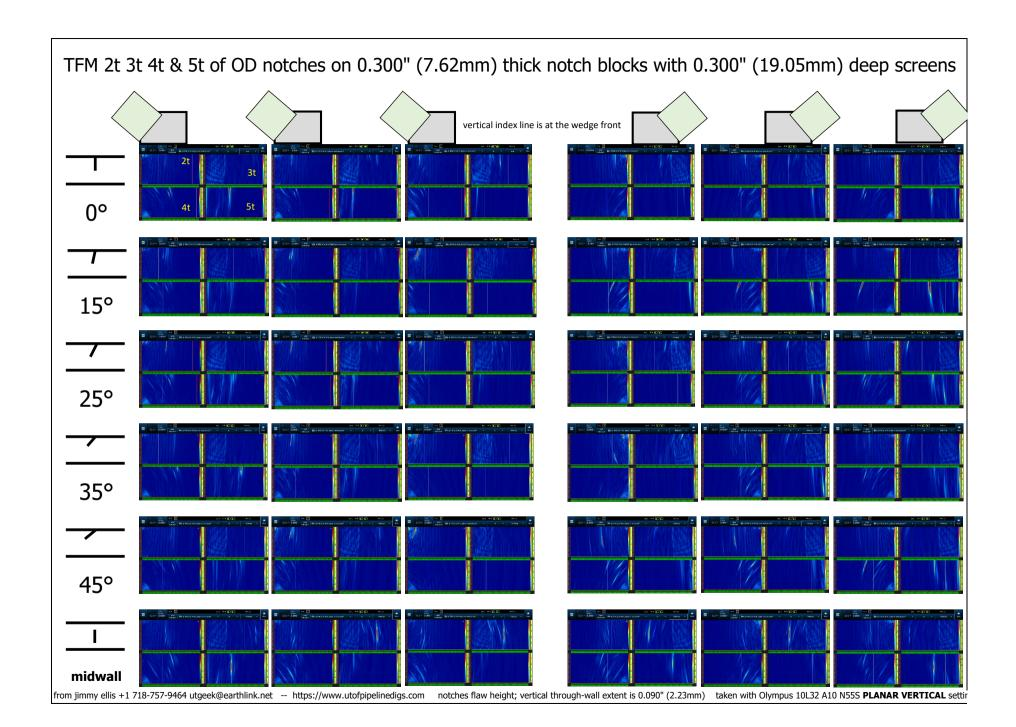
Observations for the tt **spherical** mode of ID and OD notches, with a screen 2 1/2 legs deep.
