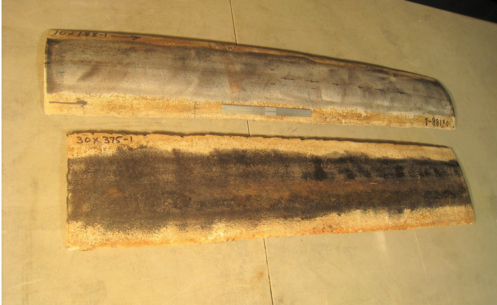
Pipe Coupons of angled notches typical sizes: 30"L x 6"W x 0.188"thk from 8x188 pipe 28"L x 6"W x 0.375"thk from 16x375 pipe
